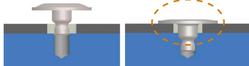
The Belleville shaped head flattens upon a simple press-in installation and draws panels together to accommodate vertical stack tolerances.
