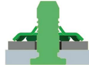
The PEM® ClampDisk® fastener can be installed onto a grooved pin to increase strength and allow installation onto any material. For more information, contact [techsupport@pemnet.com](mailto:techsupport@pemnet.com).
