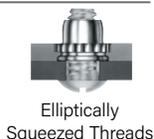
**SL™** locknuts offer a cost effective TRI-DENT® locking feature and effective prevailing locking torque — PAGE 9
