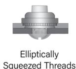
**PEM RT®** locknuts are free-running until clamp load is induced. A modified thread angle on the loaded flank provides the vibration resistant locking feature — PAGE 10
