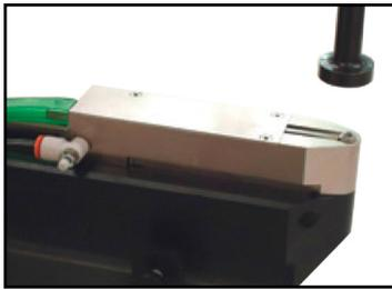
**Automatic Bottom Feed Tooling (ABFT)** for inserting nuts into at parts as well as into hard-to-reach holes. Such as those on the underside of a flange.
