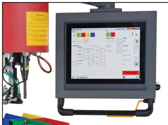
Operator control pendant can be adjusted in 6 directions.
