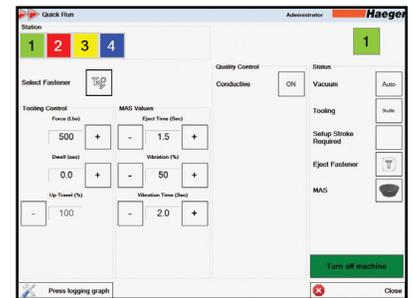
**Multi-Station:** Multi-Station is an option that allows the operator to insert more than one fastener in a program. Each station can be configured to have its own individual Force, Dwell Time and Up Travel.
