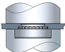
2. With installation punch and anvil surfaces parallel, apply squeezing force until the head of the nut comes in contact with the sheet material.
