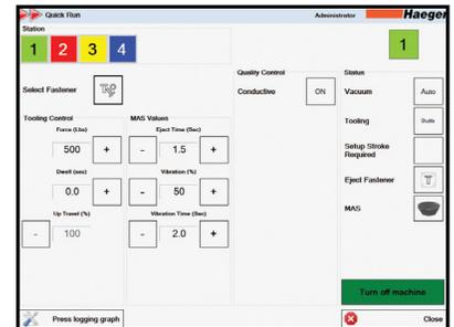
**Multi-Station:** Multi-Station is an option that allows the operator to insert more than one fastener in a program. Each station can be configured to have its own individual Force, Dwell Time and Up Travel.
