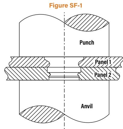
**NOTE:** To use SF or SFP fasteners as a flush-mounted pivot point, for best results, install SpotFast fastener into Panel 1 first, then place Panel 2 over fastener and squeeze again.
