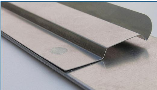
*Sheets as thin as .005" / 0.13 mm may be attached to thicker sheets using a PEM® SpotFast® fastener. The thin sheet must be panel 1 and the "L" dimension must be equal to or less than the combined panel thicknesses. Consult our Applications Engineering department for more information.*
