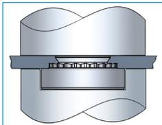
**2. With installation punch and anvil surfaces parallel, apply squeezing force until the head of the nut comes in contact with the sheet material.**
