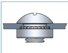
**3. Install the mating piece from the side opposite the head of the fastener.**
