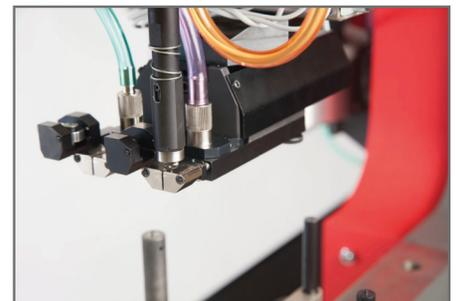
3. CLAMP TOOL AND MOVE INTO POSITION STATION 2.
