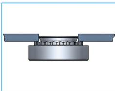
**1. Place the fastener into the anvil hole and place the mounting hole (preferably the punch side) over the shank of the fastener.**
