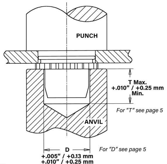
PEM miniature fasteners must be installed by a force applied through parallel surfaces. Since force must not be applied to the barrel, a cavity must be used in either the punch or anvil so that the installation force is applied to the knurled collar. "D" dimensions for the punch or anvil cavity are given in the tables on page 5.
