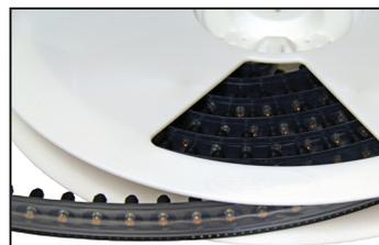
Packaged on 13" recyclable reels. Tape width is 24mm and 16mm. Pitch is 16mm and 12mm. Reels conform to EIA-481.
