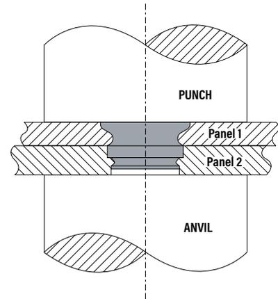
**NOTE:** To use as a flush-mounted pivot point, for best results, install SpotFast® fastener into Panel 1 first, then place Panel 2 over fastener and squeeze again.
