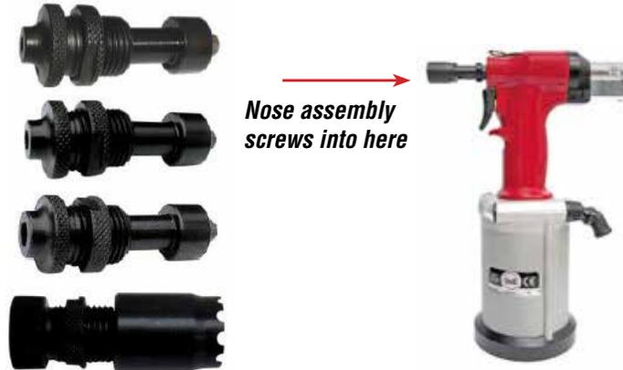
*Nose assembly screws into here*
