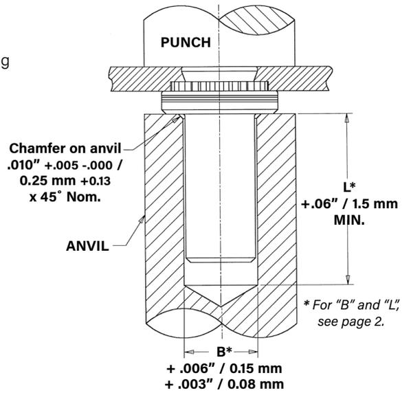
Installation Tooling - B and BS Nuts
