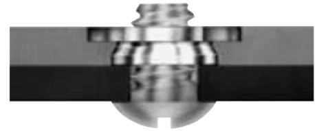
PEMSERT® flush nuts are installed easily by squeezing them into a round hole in metal sheets. They can be installed before bending and forming to provide threads in places which would be inaccessible for installation after chassis are formed. The hexagonal head along with the proven PEM® self-clinching design ensures high axial and torsional strength.
